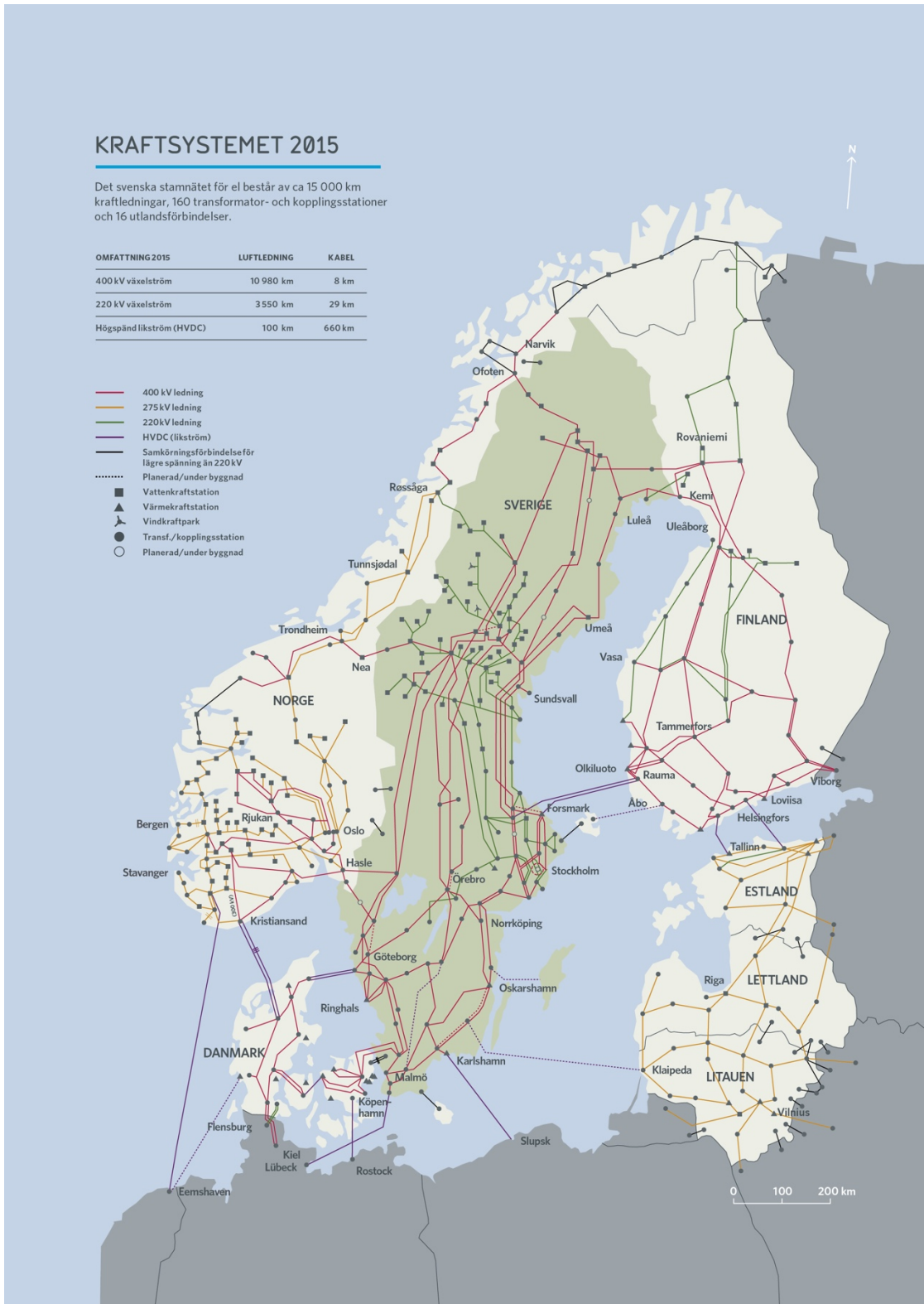
Figure 2.4. Nordic Transmission system [7].
